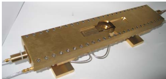
Fig. 1: Photograph of the implemented exposure device for GSM 1800MHz
